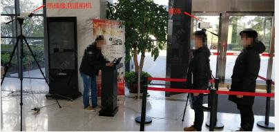
Convenient deployment: human body temperature measurement thermal imaging camera + black body + ordinary PC constitutes a small temperature measurement station
