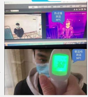
Safety: non-contact thermal imaging temperature measurement to avoid cross infection risk
