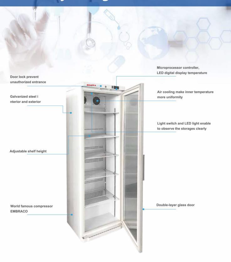
Innova pharmacy refrigerator classic is high intelligent and advanced refrigerant system which can ensure storage at 2°C~8°C. Microprocessor digital display is for easy reading and forced air cooling ensures an uniformity temperature. The controller's operation is much easiler.
