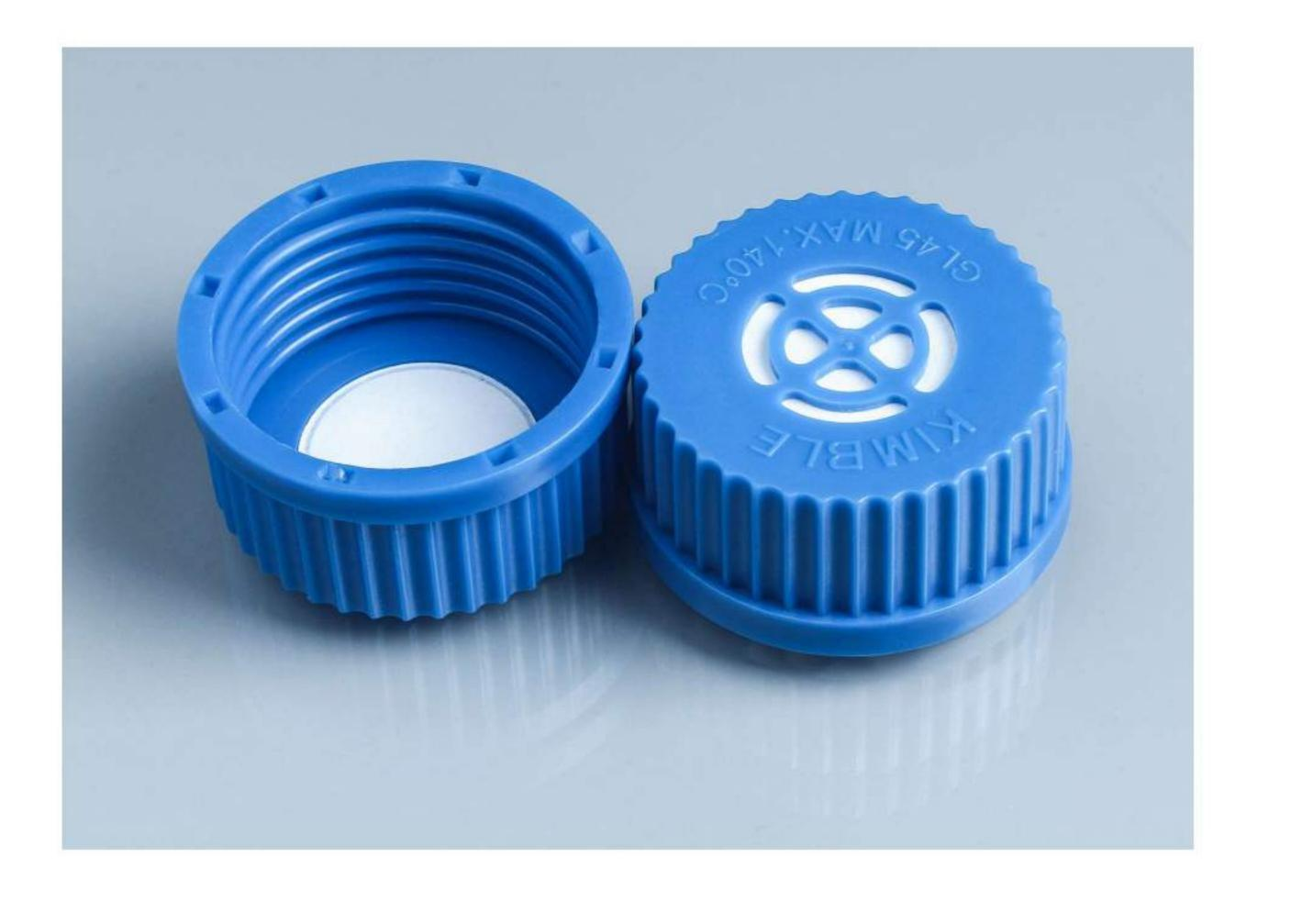
• Ingenious design inside the cover to facilitate the internal PTFE breathable membrane cell culture internal fit using custom PTFE sheet, fit without leakage of internal gasket selection of special silicone pads, to prevent the fall of the use of more worry
