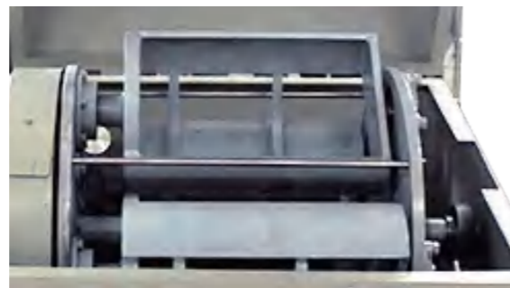
Horizontal Planetary Mechanism Gravity force and planetary force play a dual role of anti-subsidence
