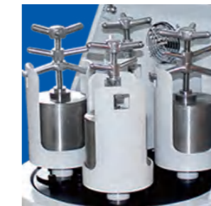
Matched with 4 mill pots of 1L volume each or Matched with 4 vacuum jars of 0.5L volume each
