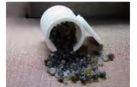
PTFE mill jar can be matched with agate balls
