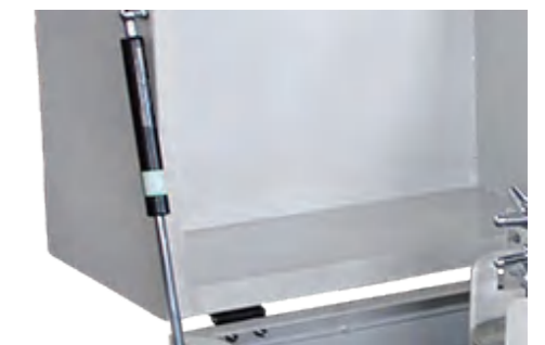
Pneumatic Rod Support force is constant in process of running with appropriate damping, safe and convenient to operate.
