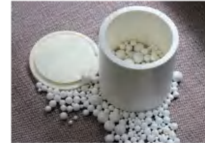
Zirconia mill jar can be matched with zirconia balls
