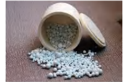
Alumina mill jar can be matched with alumina balls
