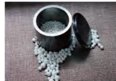
Tungsten carbide mill jar can be matched with zirconia balls
