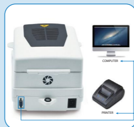
RS232 interface Which connect to Computer and Printer
